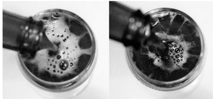
Figure 6. More constructal design of turbulence in a glass of dark beer. The momentum from the falling liquid is transferred more effectively to the body of stationary liquid by a design of eddies regularly spaced around the rim. The bubbles gather on the surface only above the regions that correspond to downward flow.
