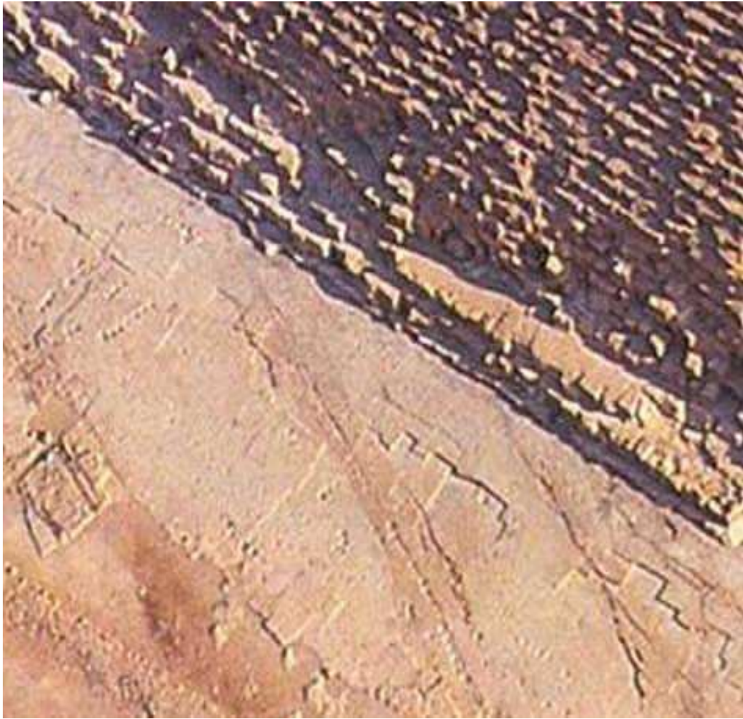
Figure 21: Aerial shot of Cheops' "temenos", showing the quarry exploitation of the blocks according to the secondary fracturing (diagonal to the axis of the fold)
